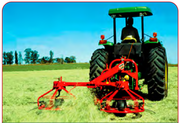
Rake rotates when working and locks when lifted
