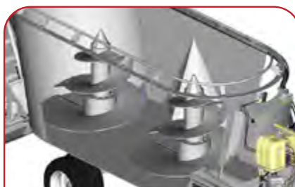
Double auger for a homogeneous mix
