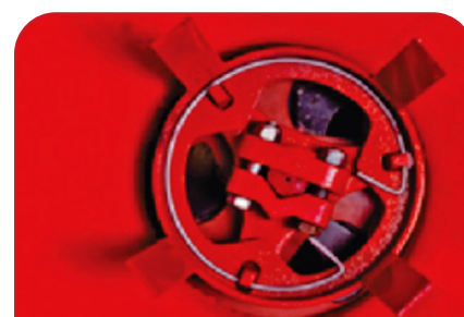
Shaker with oscillating system
